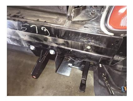
Figure 2: Hook mounted on driver side
